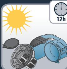
**EN** Once a week, wash the filter with clear water and clean the dust container and the cyclone manually.
