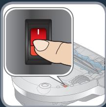
**EN** Turn the robot upside down and turn the robot OFF ( O ).
