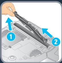
**EN** Remove the brush guard, and pull out the brush.
