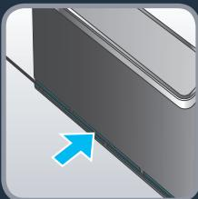
**EN** Plug the adaptor to the power jack on the side of the base. Hide the excessive cord on the back of the base, in the space provided for that purpose. Only use the charger provided with the robot: do not use universal chargers.
