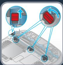
**EN** Unlock the brush guard using the 4 lockers.
