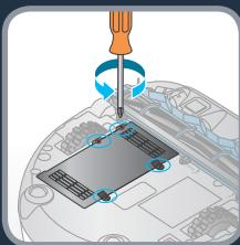
**EN** With a screwdriver, unscrew the battery compartment lids. Disconnect the battery and remove the battery from the robot.
