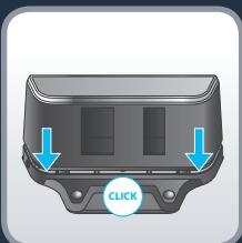
**EN** Clip the two parts of the docking station together.
