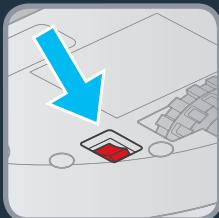
**EN** Turn the robot upside down and turn the power switch ON (I). You will see LED lights blinking on the robot's dashboard for few seconds.
